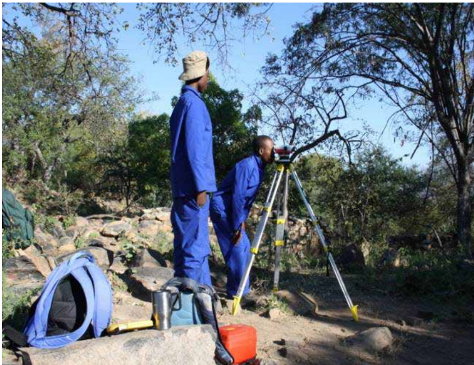
Figure 3: University of Botswana students using dumpy level to take excavation levels at one of the enclosures during the 2010 field school (Photograph by Mothulatshipi).
